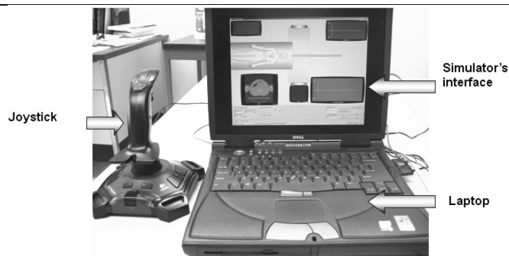
Fig. 1. Illustration of CT table simulator. which is compose of joystick and laptop.
